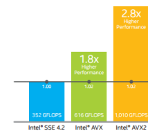
Figure 1. Measuring performance on the same processor using Linpack* benchmarks shows substantial increases from Intel® Streaming SIMD Extensions 4.2 (Intel® SSE 4.2) to Intel® Advanced Vector Extensions (Intel® AVX) and from Intel AVX to Intel® AVX2, with up to 2.8x the GFLOPS throughput when comparing Intel SSE 4.2 to Intel AVX2. 2
